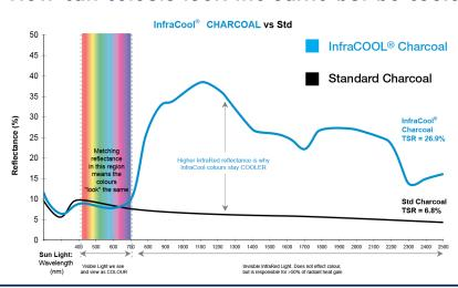
This chart shows the "Spectral Reflectance" of InfraCOOL® Charcoal vs Standard Charcoal. Its the way we measure reflectance of sun light across the full spectrum. The rainbow portion depicts the wave lengths of light in the "visible spectrum" which determines colour as we see it.
